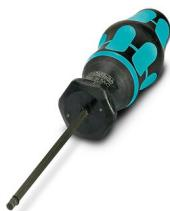
Torque screwdriver, with preset torque of 2.0 Nm and 4 mm hexagonal drive for the pressure nut of the fast connection
